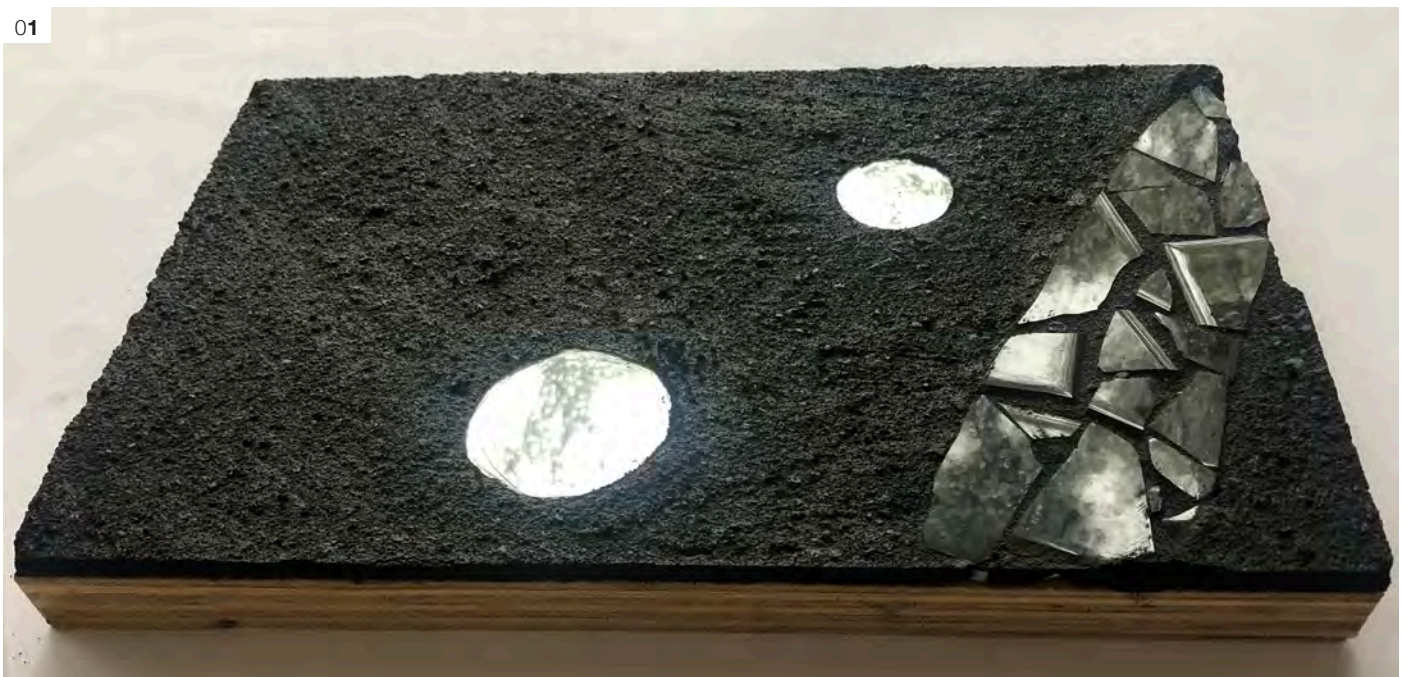
Images: 01 prototype mockup, black cement render with an array of 30mm and 60mm mirrored spots and fragments of gloss black ceramic tile mosaics
