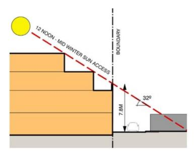
The benefits of this resolution are that properties on the south side of Chesterfield Lane will have less overshadowing effects. The 32 degree angle correlates with the angle of the sun at noon on the winter solstice.
