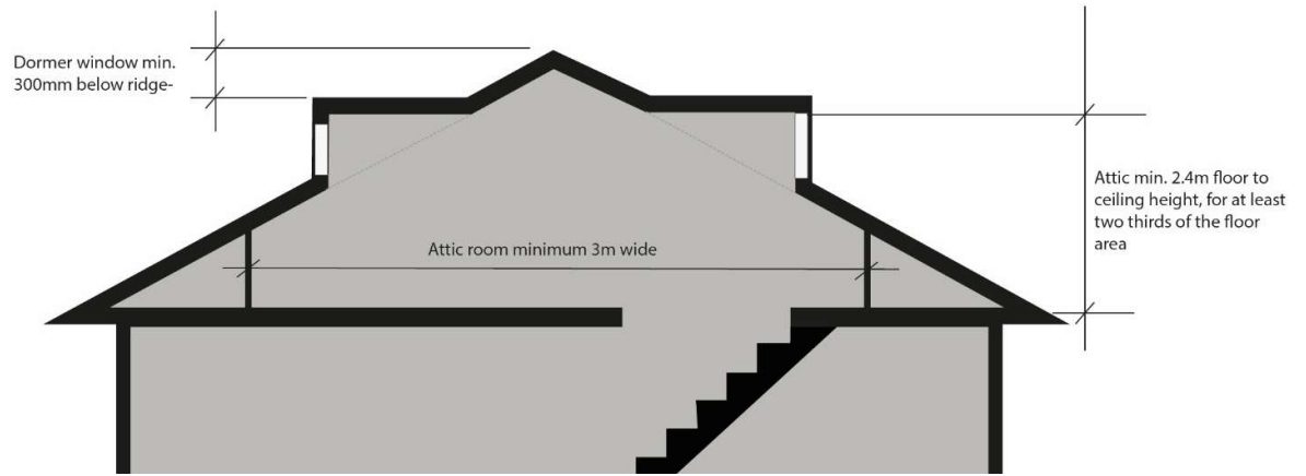
Figure 21 Pitched roof minimum attic dimensions
