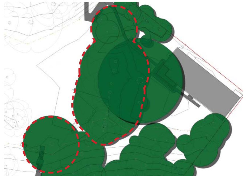
Trees recommended for removal : These trees are Camphor Laurels which have soft wood and are likely to rapidly break down. 7 of the trees are identified as being an immediate risk in the Vegetation Management Plan, due to trunk decay and disease. The rest are noted for future removal since these are environmental weeds. All trees are in a copse with inter-twined roots. Thus it is advisable to remove the whole tree line at one go for safety reasons. The removal in turn will help provide space for the Historic Fig to flourish as well as provide much needed sunlight for the proposed lawn areas.
