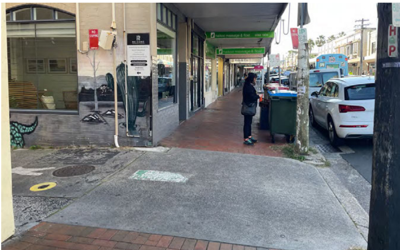
Site image: The lane crossing at Cables Lane does not reflect pedestrian priority – potential for continuous footpath
